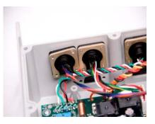
4. Connect harness to P2 on the Main circuit board. Match locking tab.
