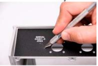
5. Attach harness to bottom of housing with screws and screw plate. Check that connector is oriented correctly.
