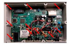
10. Position the radio antenna up from the radio, next to J901.
