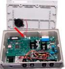
2. Remove screws from Main circuit board and existing Option circuit board.
