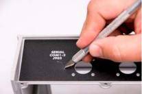
5. Cut hole for radio connector.
