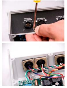
10. Place new Option circuit board in housing while connecting P1 to J1 on the Main circuit board.
