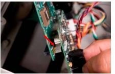
11. Move circuit boards back into position in the housing, lining up the Datakey keyceptacle with the housing. Attach circuit boards to the housing with screws.
