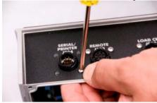
5. Place Option circuit board in housing while connecting P1 to J1 on the Main circuit board (see diagram). Attach to the housing with screws.
