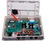
2. Cut holes for J904 connector in the bottom overlay.
