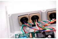
4. Place Option circuit board in housing while connecting P1 to J1 on the Main circuit board.
