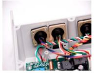
8. Place new Option circuit board in housing while connecting P1 to J1 on the Main circuit board.
