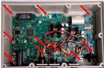
5. Move circuit boards up slightly to allow the Datakey keyceptacle to clear the housing.
