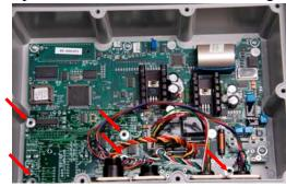
3. If needed, remove the existing J904 harness from the bottom of the housing.
