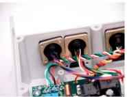
6. Place Option circuit board in housing while connecting P1 to J1 on the Main circuit board.
