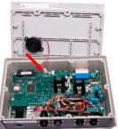
2. Remove screws from Main circuit board and existing Option circuit board.
