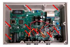
3. If needed, remove the existing J905 harness from the bottom of the housing.
