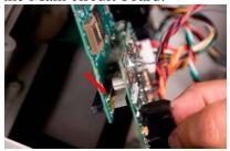
9. Move circuit boards back into position in the housing, lining up the Datakey keyceptacle with the housing. Attach circuit boards to the housing with screws.
