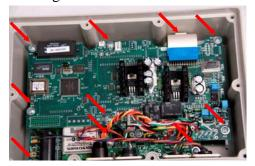
12. Position the radio antenna up from the radio, next to J901.
