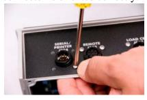
9. Connect Option circuit board to the Main circuit board, P1 to J1.
