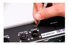
7. Move circuit boards up slightly to allow the Datakey keyceptacle to clear the housing.
