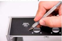
6. Cut hole for radio connector.
