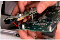
12. Add Display to board stack with Main board, P1 to J3. Hold with standoffs line up
