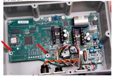
3. Place Option circuit board in housing while connecting P1 to J1 on the Main circuit board.
