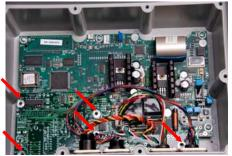
5. Position the radio antenna up from the radio, next to J901.
