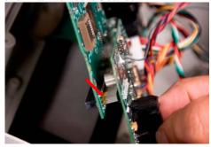
4. Move circuit boards back into position in the housing, lining up the Datakey keyceptacle with the housing. Attach circuit boards to the housing with screws.
