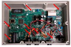
3. Place new Option circuit board in housing while connecting P1 to J1 on the Main circuit board.
