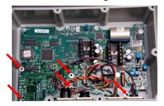
8. Position the radio antenna up from the radio, next to J901.
