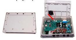
2. If the indicator contains an Option circuit board, remove the screws from the Option circuit board. Remove the Option circuit board from the housing.
