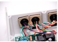
6. Place Option circuit board in housing while connecting P1 to J1 on the Main circuit board.
