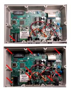
10. Position the radio antenna up from the radio, next to J901.
