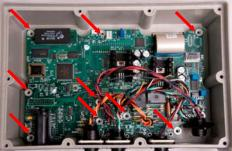
3. Place new Option circuit board in housing while connecting P1 to J1 on the Main circuit board.
