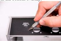
5. Cut hole for radio connector.
