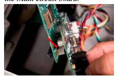
11. Move circuit boards back into position in the housing, lining up the Datakey keyceptacle with the housing. Attach circuit boards to the housing with screws.
