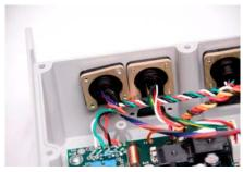
10. Place new Option circuit board in housing while connecting P1 to J1 on the Main circuit board.
