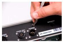
6. Move circuit boards up slightly to allow the Datakey keyceptacle to clear the housing.
