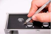
6. Cut hole for radio connector.
