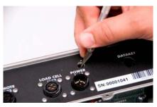
7. Move circuit boards up slightly to allow the Datakey keyceptacle to clear the housing.
