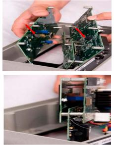
13. Move circuit boards back into position in the housing, lining up the Datakey keyceptacle with the housing. Hold keypad pigtail against housing and reconnect. Attach circuit boards to the housing with screws.
