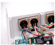
8. Place new Option circuit board in housing while connecting P1 to J1 on the Main circuit board.
