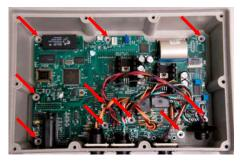
3. If needed, remove the existing J904 harness from the bottom of the housing.
