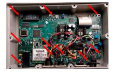
10. Position the radio antenna up from the radio, next to J901.
