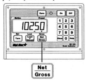
Press the [NET/GROSS] key if in the NET or LOAD/UNLOAD mode.
