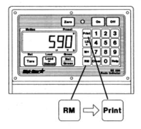
The [PRINT] key causes the unit to return to the normal weighing modes.
