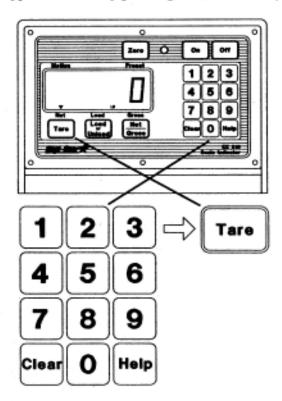
The preload tare feature is useful for weighing containers after they have already been loaded. If the weight of the container is known, this "tare weight" could be preloaded into the scale and the net weight will be displayed. The "tare weight" is also sent to the printer.
