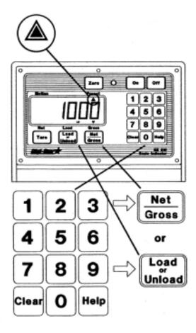
Once the preset has been entered, the display can show the weight data in three (3) different "display modes". The three display modes are:
