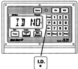
The identification number is cleared by pressing the [CLEAR] key followed by pressing the [ID #] key
