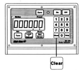
At this time, a new preset can be entered or by pressing the [CLEAR] key a second time (with a flashing zero " 0" shown on the display) the scale will return to weighing.
