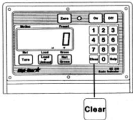
Step 3) Use the numeric keypad to select a pre-alarm weight.
