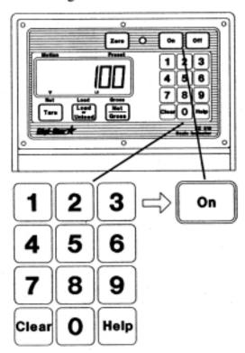
Step 4) Press the [ON] key. The display will advance to the next setup value.
